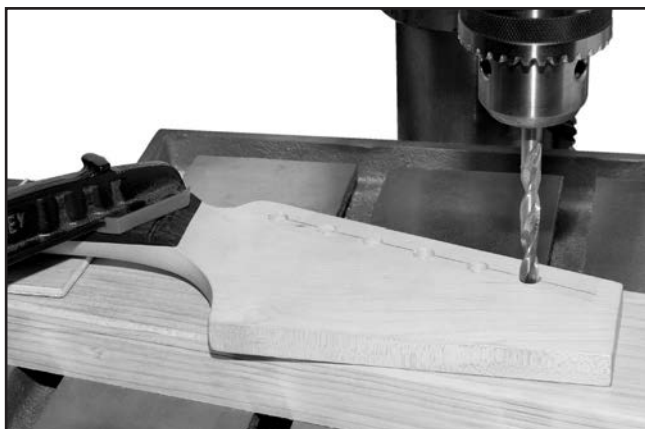
Figure 10. Drilling the pegholes.
