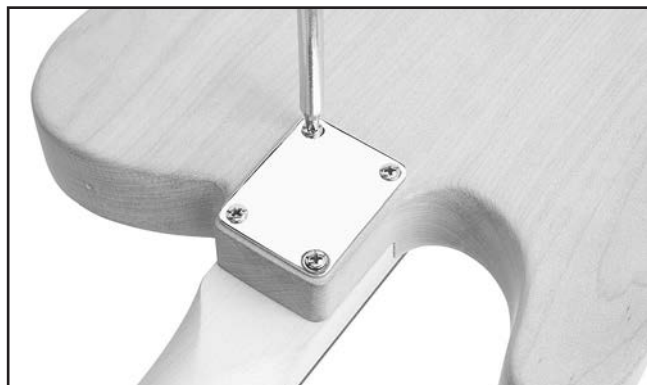
Figure 20. Fastening neck to body.
