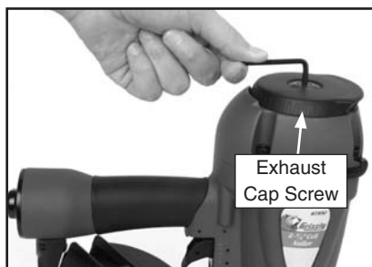
Figure 10. Loosening the exhaust cap screw.
