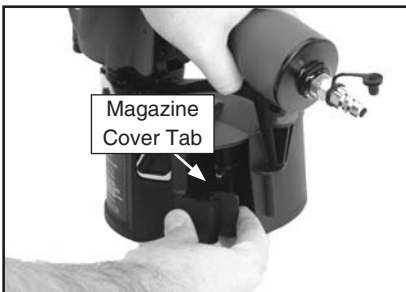
Figure 3. Opening the magazine: Model H7949/H7950.
