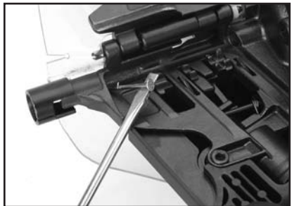
Figure 14. Prying a jammed nail from the driving hole.
