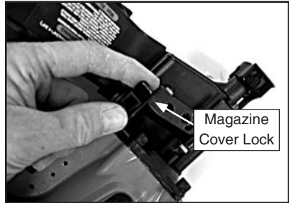
Figure 7. Unlatching the magazine cover lock: Model H7951.
