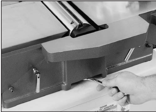
Figure 3. Removing nut on bearing block stud.
