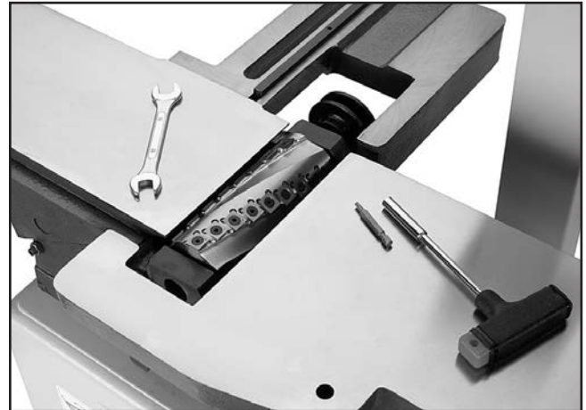
Figure 5. Spiral cutterhead installed.
