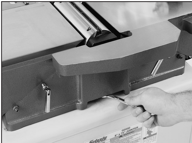
Figure 4. Removing nut on bearing block stud.
