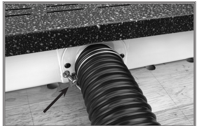
Figure 2. Dust port connected to dust collection system.
