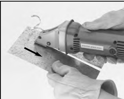
Figure 4. Cutting small stock.
