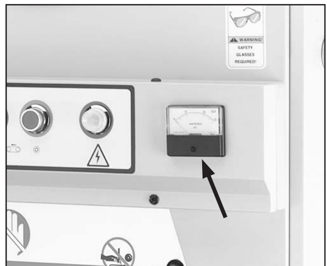
Figure 20. This is the load meter.
