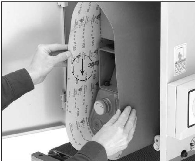
Figure 13. Place belt over the three belt rollers to install. Make sure arrows on inside of belt point in the direction of rotation.
