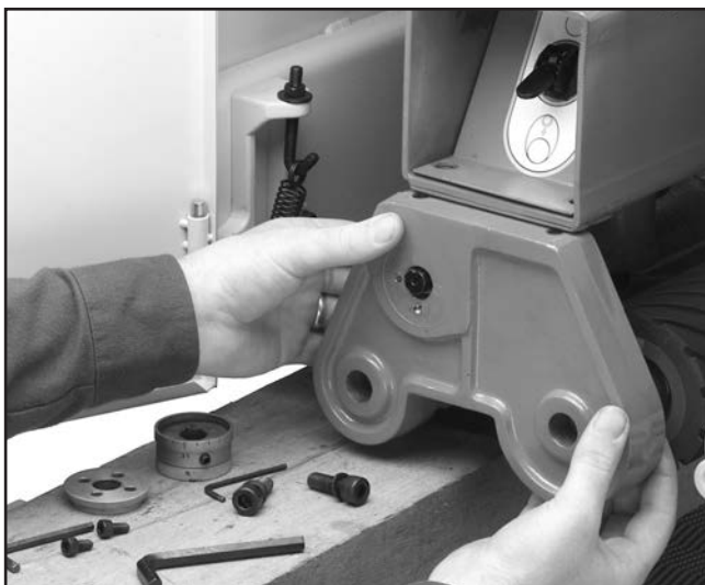
Figure 36. Work the casting off the roller shafts.
