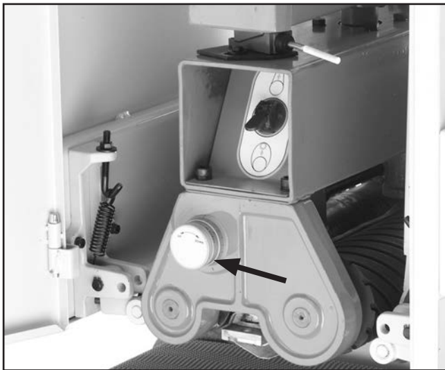
Figure 11. Use this knob to raise/lower the platen.
