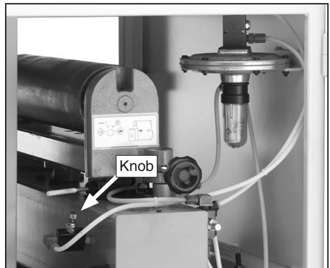
Figure 27. Use the knob on this valve to control oscillation speed.
