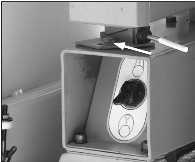
Figure 29. Loosen these bolts to adjust the limit switch position.
