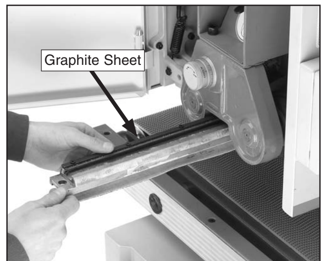
Figure 10. Install the platen with the graphite sheet on the left-hand side.
