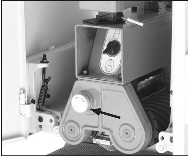
Figure 21. The scale on this knob tells you how far you have moved the platen.
