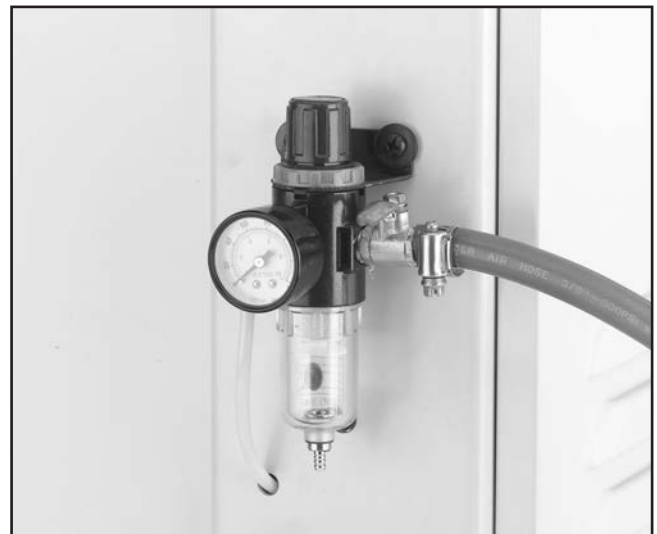
Figure 12. Secure air hose with a hose clamp.
