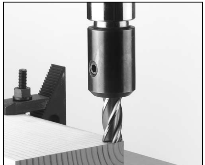
Figure 23. Cutter just touching workpiece.
