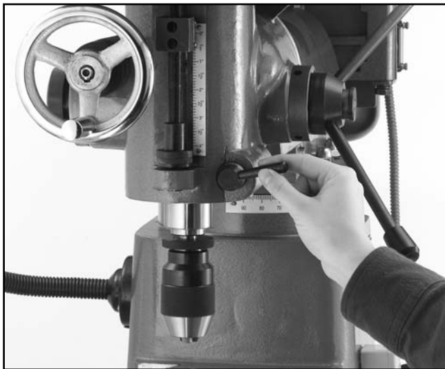
Figure 8. Secure quill with this lever.
