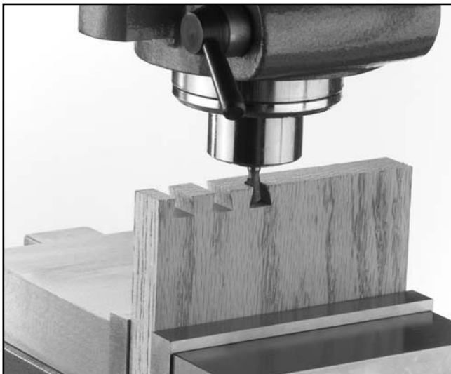
Figure 23. Cutting very accurate dovetails.
