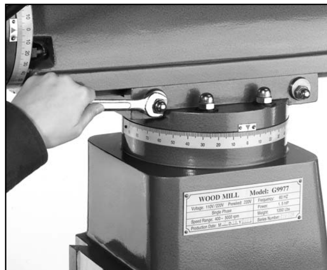
Figure 13. Loosen locking bolts.
