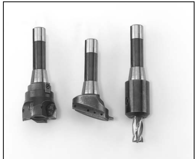
Figure 22. Various cutting tools for facing.
