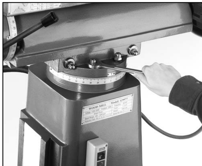
Figure 12. Loosen hex nuts to swivel head.
