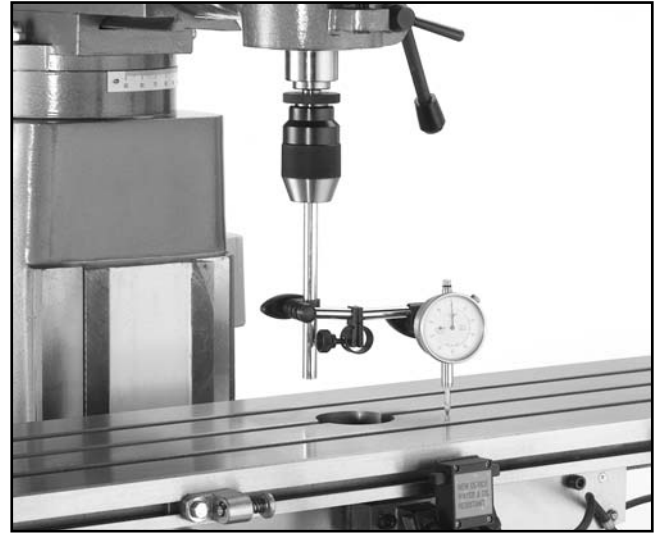
Figure 11. Indicator mounted to test head.
