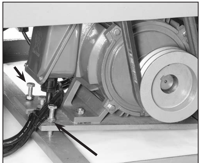
Figure 23. Motor mount adjustment bolts.
