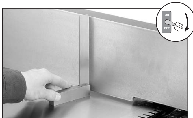
Figure 65. Setting the fence to 90° (cutterhead guard moved away for clarity).
