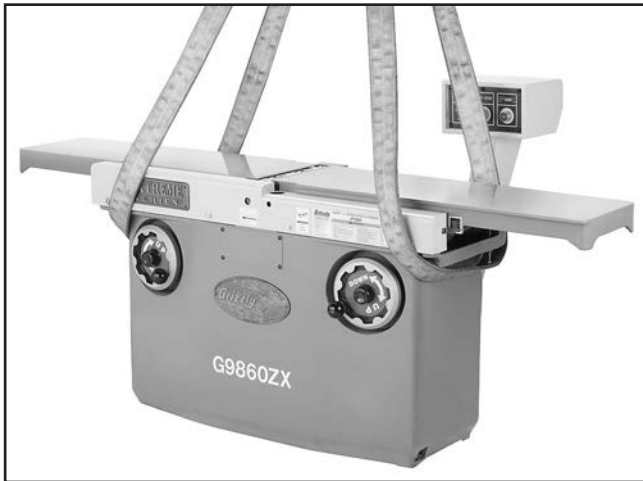
Figure 16. Lifting straps properly positioned.
