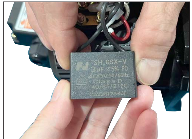
Figure 88. Pump start capacitor.
