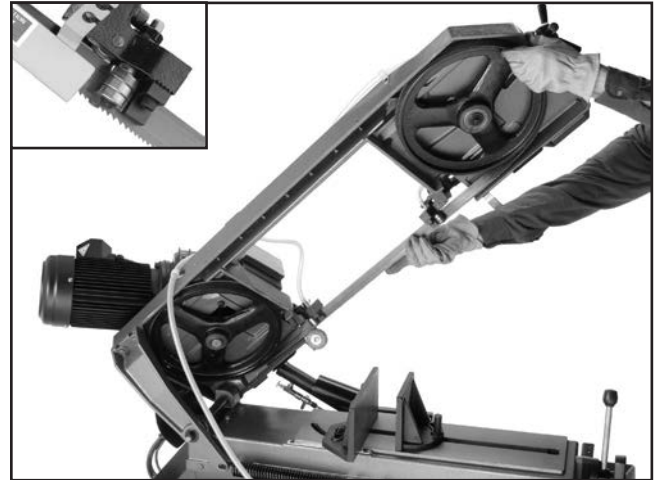
Figure 39. Typical blade installation.
