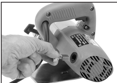
Figure 9. Replacing a motor brush.
