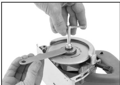
Figure 7. Replacing the diamond blade.
