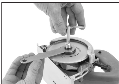
Figure 2. Attach the cutting blade.
