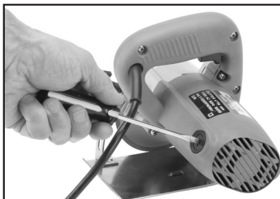
Figure 8. Removing a brush cap.
