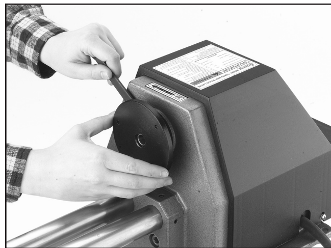
Figure 11. Installing the faceplate.
