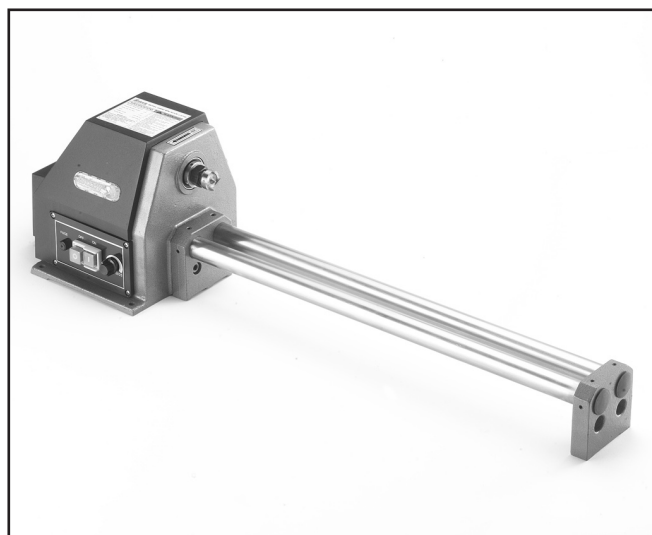
Figure 6. Guide rails installed.
