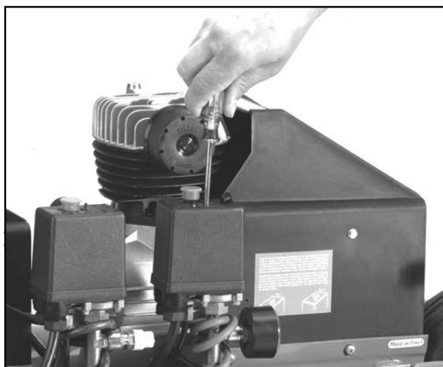
Fig 10. Removing pressure switch cover.
