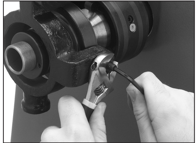
Figure 10. Tightening yoke setscrews.
