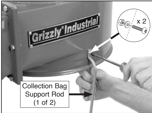
Figure 10. Attaching collection bag support rods to collector.
