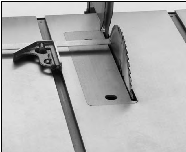
Figure 21. Adjusting blade to miter slot.
