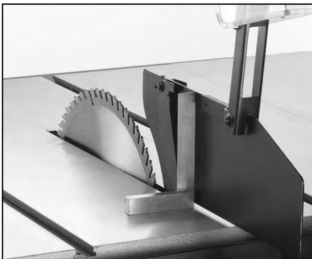
Figure 13. Guard assembly square to table.
