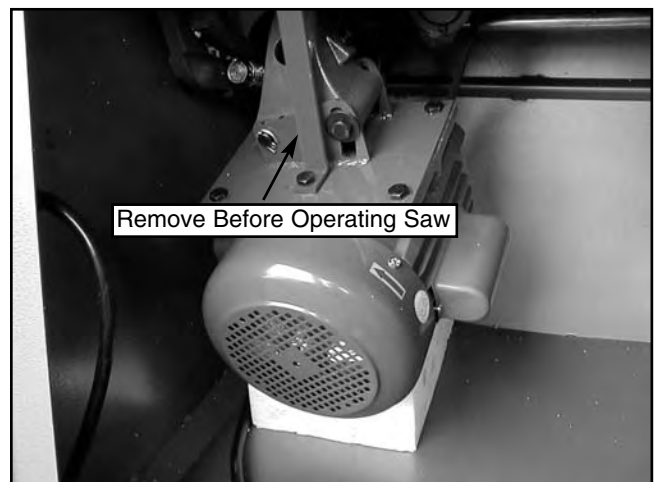
Figure 10C. Remove motor bracket.
