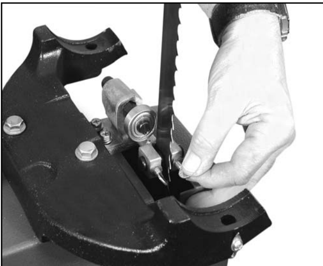
Figure 4. Installing blade guide assemblies.
