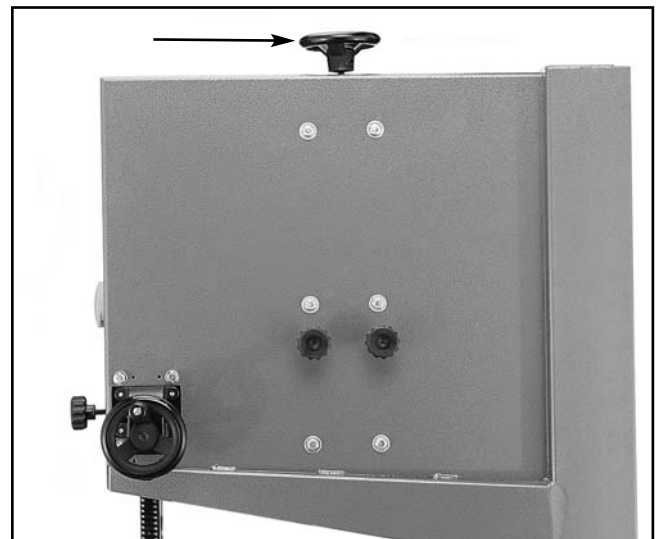
Figure 27. Tension control knob.
