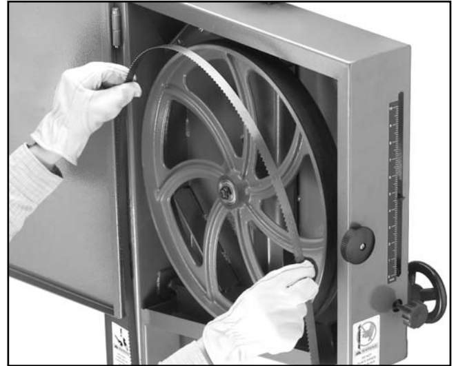
Figure 9. Fitting blade over upper wheel.
