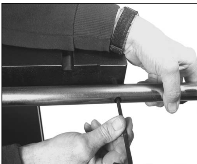
Figure 7. Securing the rail to the table.
