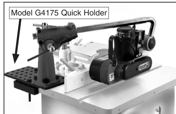
Figure 14. Typical power feed mounting using optional Model G4175 Quick Holder.
