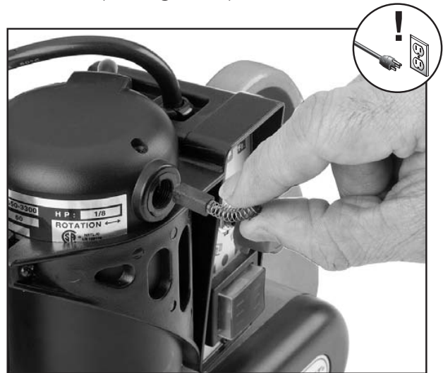
Figure 29. Replacing brush set.
