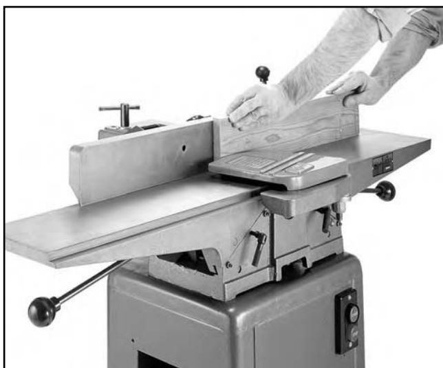
Figure 25. Operator position for edge jointing.
