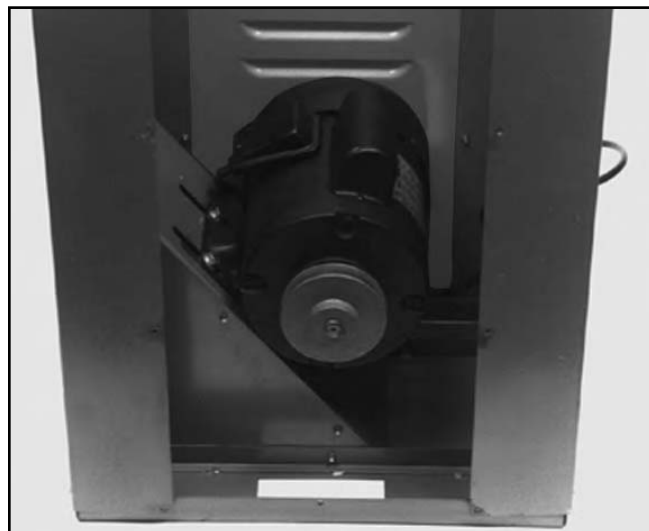
Figure 7. Attaching the motor.
