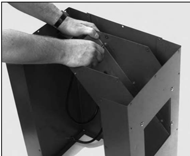
Figure 5. Attaching the dust chute base.
