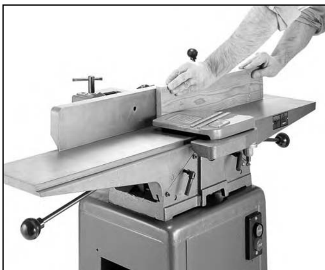
Figure 25. Operator position for edge jointing.
