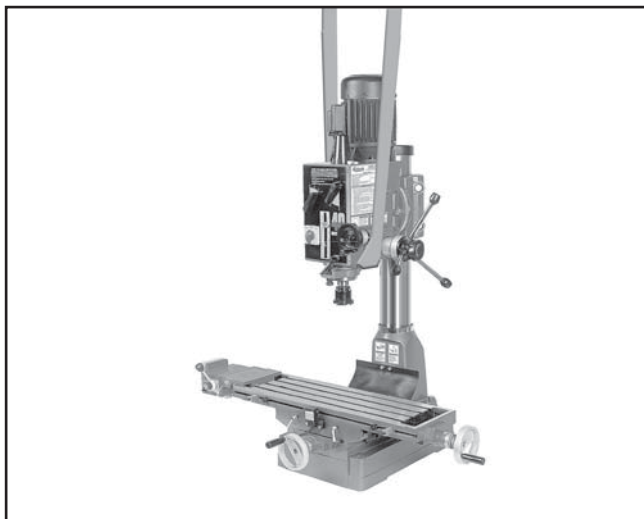
Figure 9. Typical lifting strap position.
