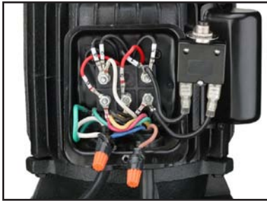
Figure 76. 110V motor wiring.
