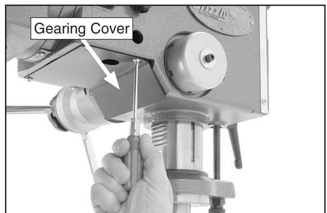
Figure 39. Removing gearing cover.
