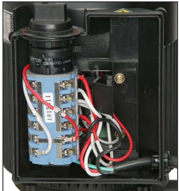
Figure 28. Motor switch (front view, G1096).
