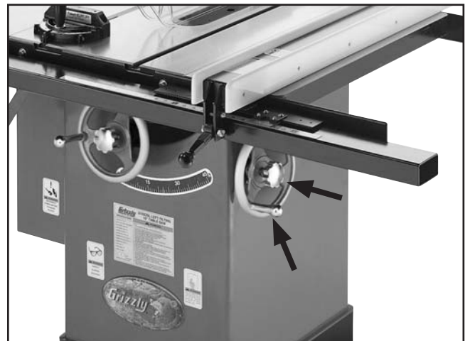
Figure 24. Handle and lock knob installed on handwheel.
