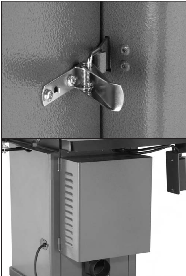
Figure 22. Motor cover installed on stand.
