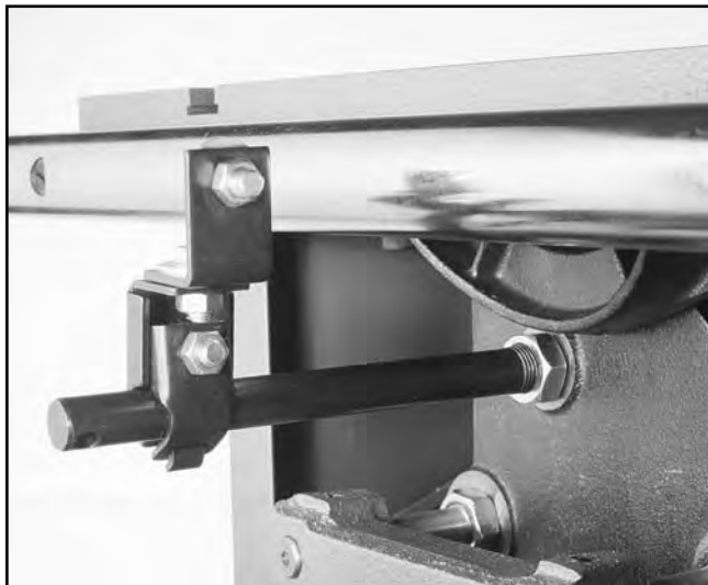
Figure 25. Installing blade guard.
