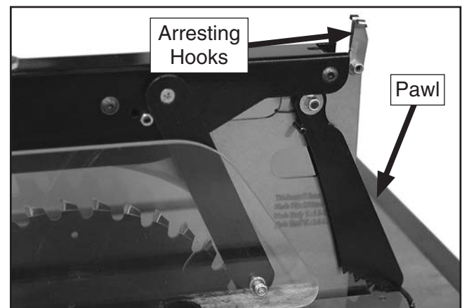
Figure 42. Pawls in resting position.
