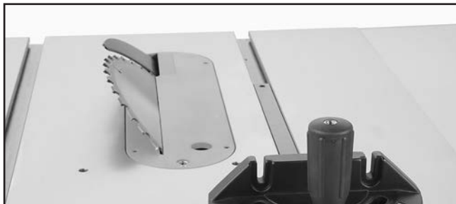
Figure 49. Blade tilted to 45° for bevel cutting on a typical table saw.
