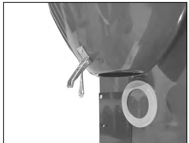
Figure 23. Dust collector dump chute.
