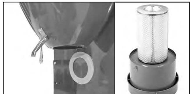
Figure 32. Dust collector service.
