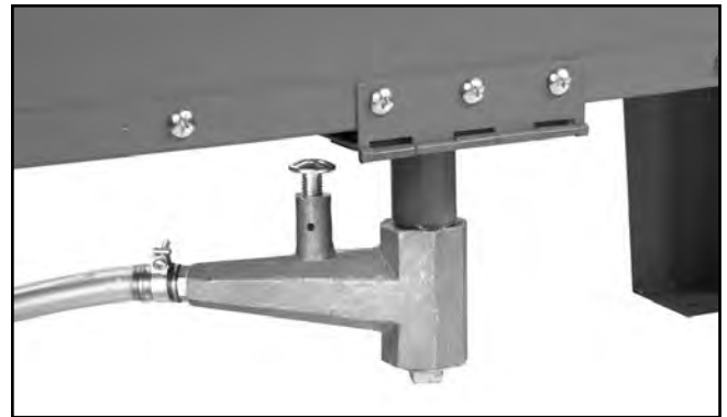
Figure 8. Hopper chute w/metering valve installed
