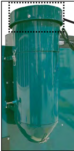
Figure 45. Dust collector unit.
