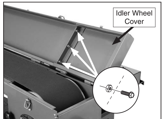
Figure 22. Platen cover connection.
