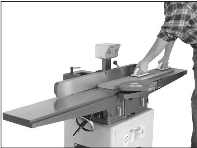
Figure 32. Typical surface planing operation.
