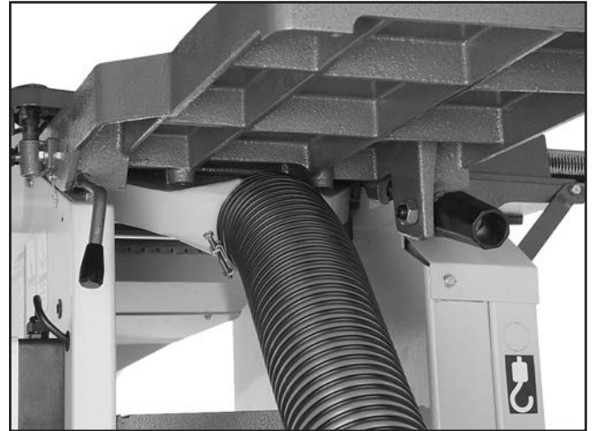
Figure 15. Dust hose attached to jointer dust port.
