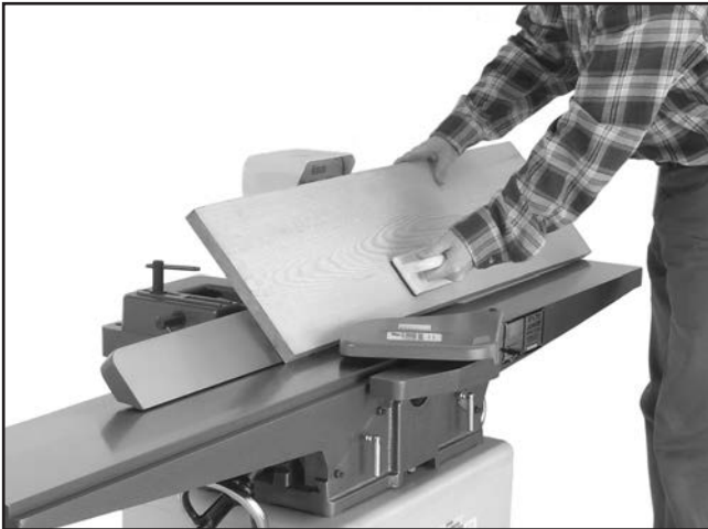
Figure 36. Typical bevel cutting operation.
