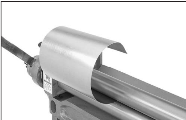
Figure 22. Repositioning workpiece to remove the initial flat.
