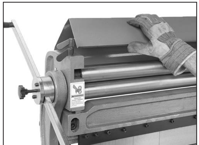
Figure 16. Slip roll preparation.
