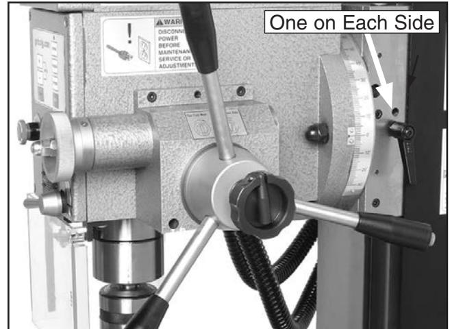
Figure 32. Headstock ball oiler locations.
