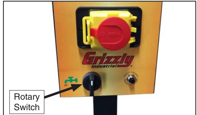
Figure 1. G0613 control panel.
