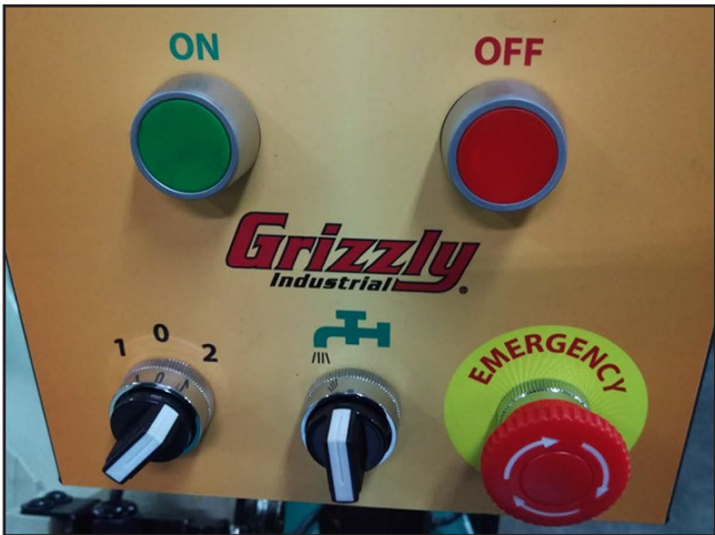
Figure 14. G0614 control panel.
