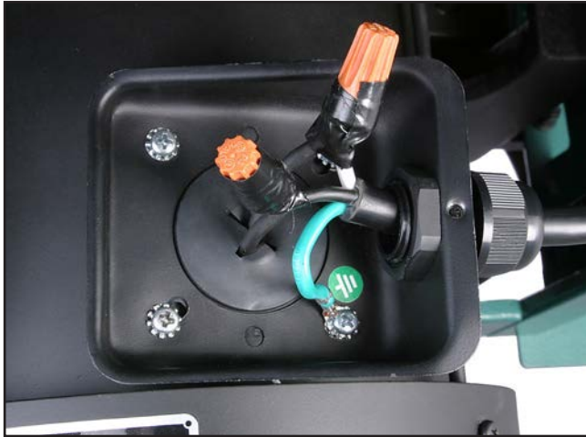
Figure 154. G0605X1/G0696X motor junction box.
