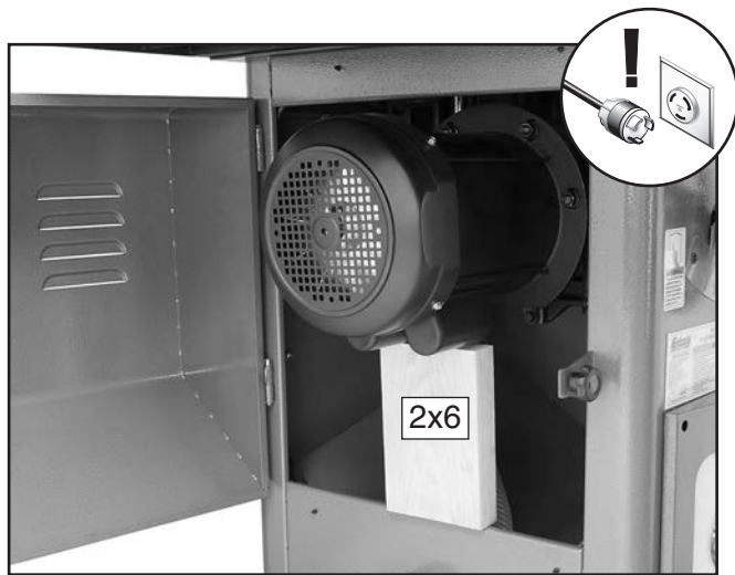
Figure 150. Motor resting on wood block.
