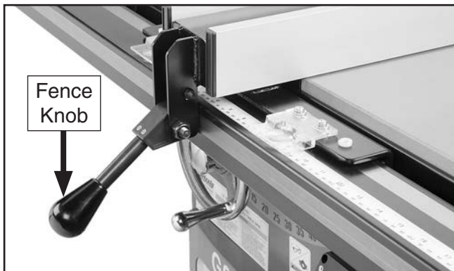
Figure 41. Fence knob installed.
