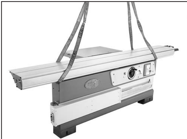
Figure 16. Installing the sliding table.
