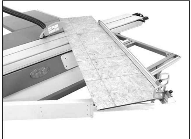
Figure 64. Example of miter cutting operation.
