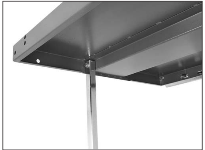
Figure 20. Support leg installation.
