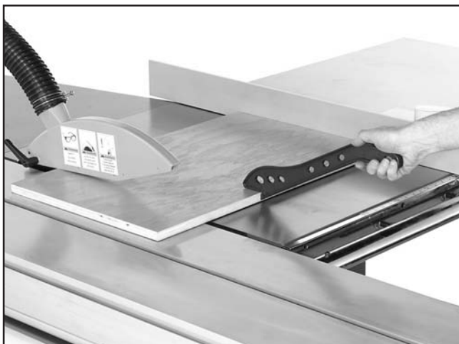
Figure 51. Traditional rip cutting.
