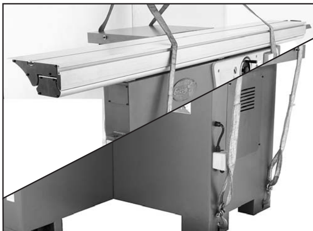
Figure 9. Lifting the saw base unit.
