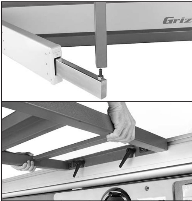
Figure 42. Installing the crosscut table.
