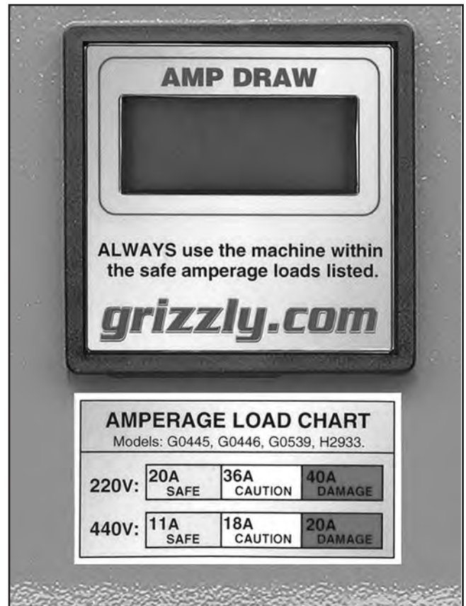
Figure 17. Typical amp draw meter and load chart.
