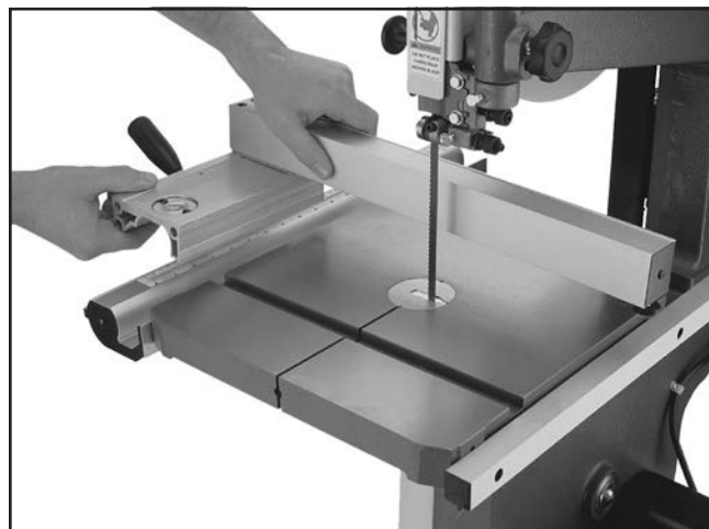
Figure 20. Placing the fence onto the rails.
