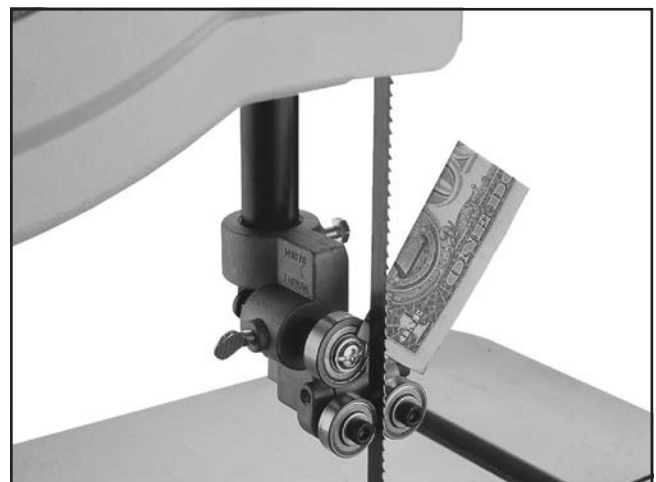
Figure 30. Dollar bill folded twice to make a quick 0.016" gauge.
