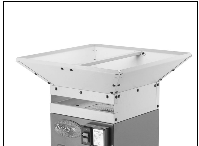
Figure 18. Collection box installed on motor cabinet.
