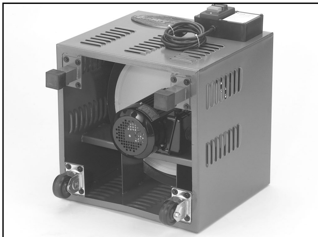
Figure 11. Casters and feet installed on motor cabinet.
