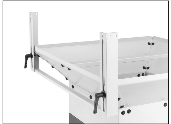
Figure 20. Curtain frame installed on curtain brackets.
