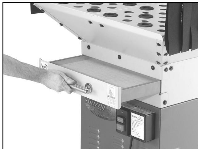
Figure 23. Sliding filter drawer into filter box.
