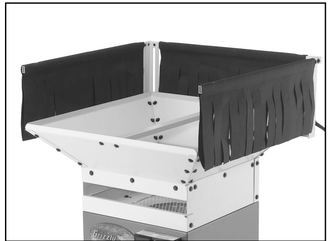
Figure 21. Curtains installed on curtain frame.
