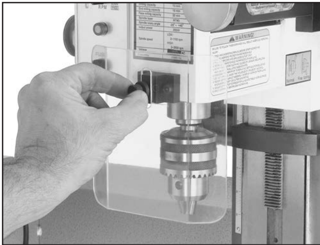
Figure 8. Attaching eyeshield to the mill/drill head.
