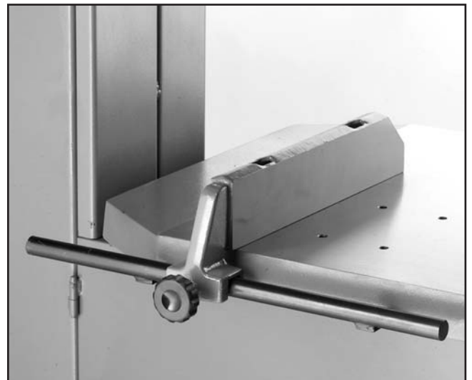
Figure 7. Fence mounted on rail.
