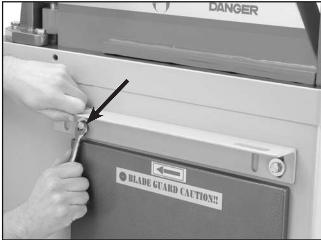
Figure 9. Attaching mounting bracket to saw.
