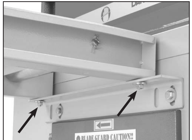
Figure 12. Roller table attached to mounting bracket.
