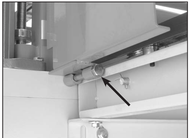
Figure 23. Left side of safety guard secured through welded bracket.
