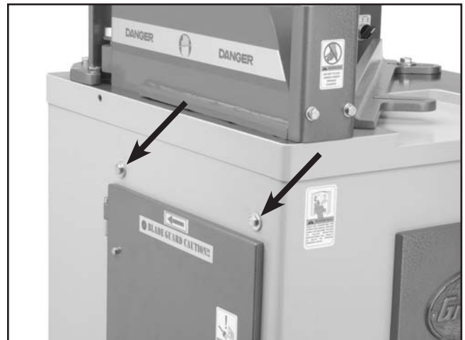
Figure 8. Bolts to be removed.
