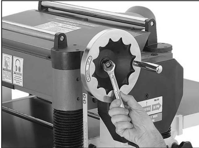
Figure 9. Installing the table height handwheel.
