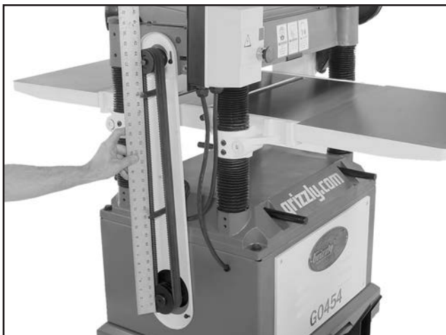
Figure 52. Checking pulley alignment.
