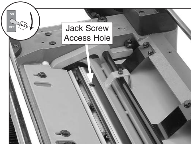
Figure 36. Jack screw access hole in the cutterhead.
