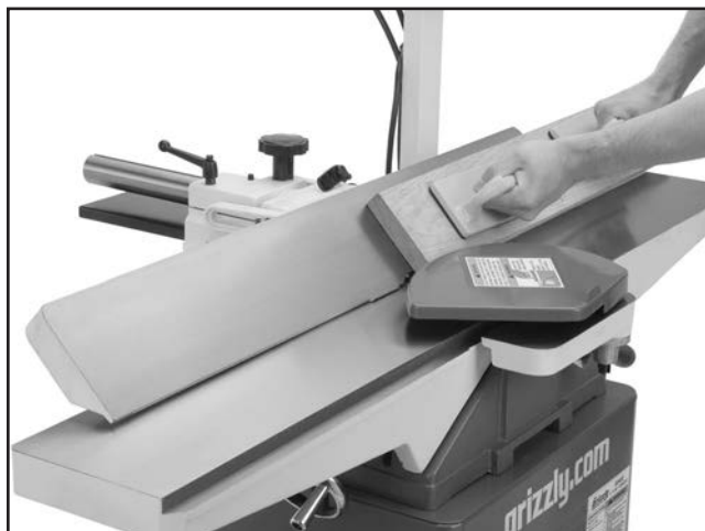
Figure 47. Typical bevel cutting operation.
