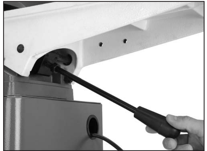
Figure 39. Adjusting infeed table height.
