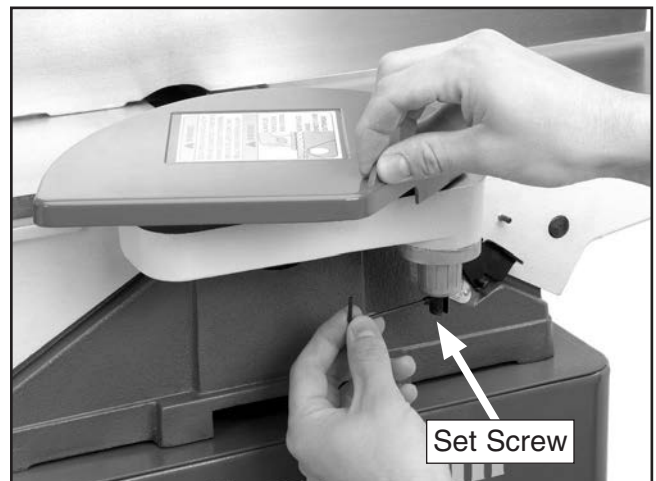
Figure 24. Re-installing set screw.
