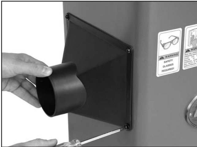
Figure 25. Dust port installation.
