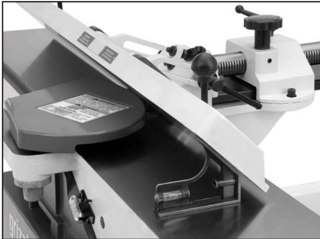
Figure 72. Adjusting fence 45° inward.
