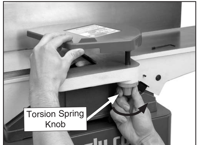
Figure 23. Setting torsion spring knob.
