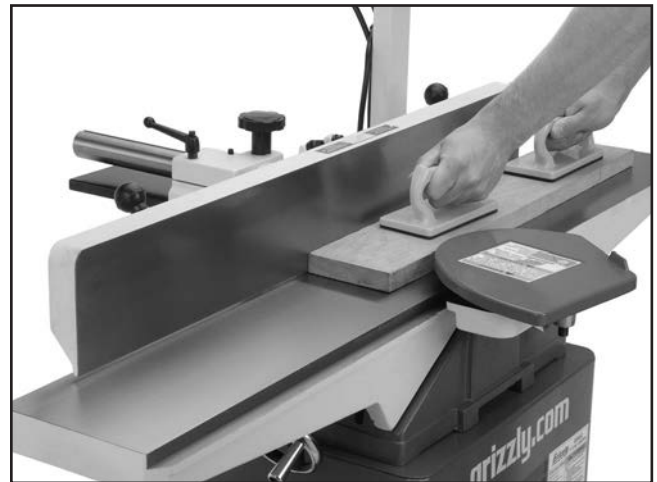
Figure 43. Typical surface planing operation.
