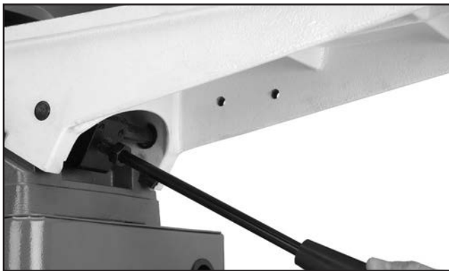
Figure 29. Installing infeed table lever.
