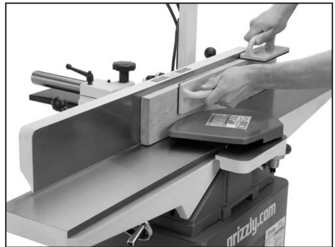
Figure 45. Typical edge jointing operation.
