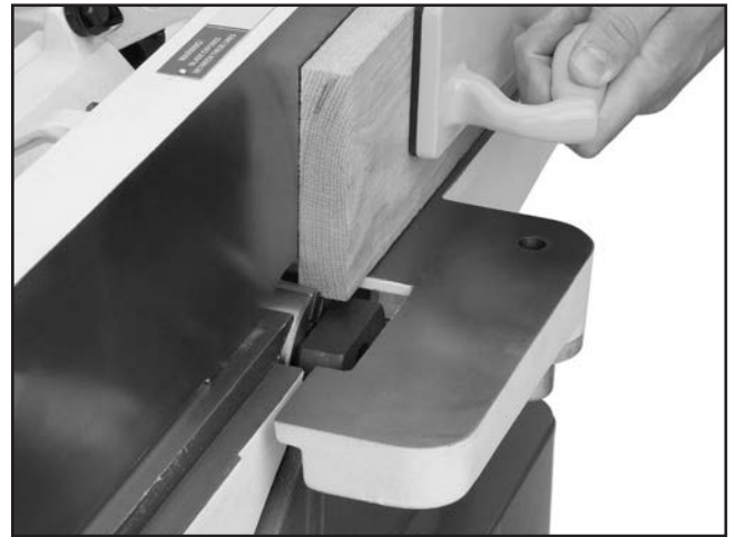
Figure 49. Typical rabbet cutting operation.
