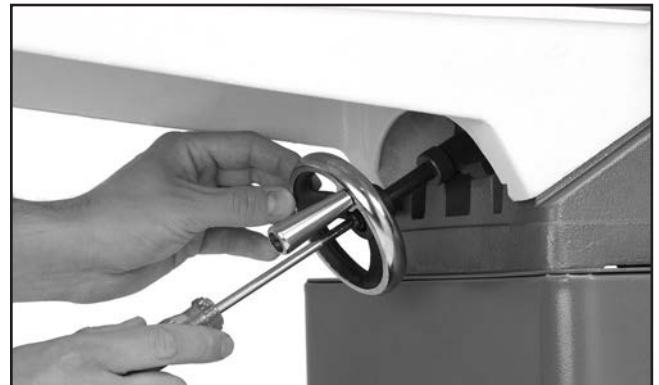
Figure 28. Securing the handwheel.
